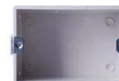
45DH118 118 Flush mounting box, Size: 99.5x65x47.5mm, Mounting centres: 83.5mm
