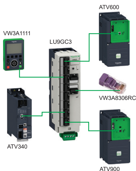
Example of multipoint screen architecture
