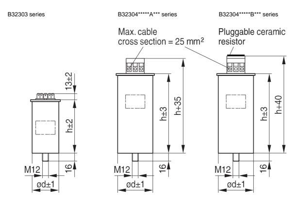
Torque = 10 Nm, Toothed washer J12 DIN 6797, Hex nut BM 12 DIN 439
