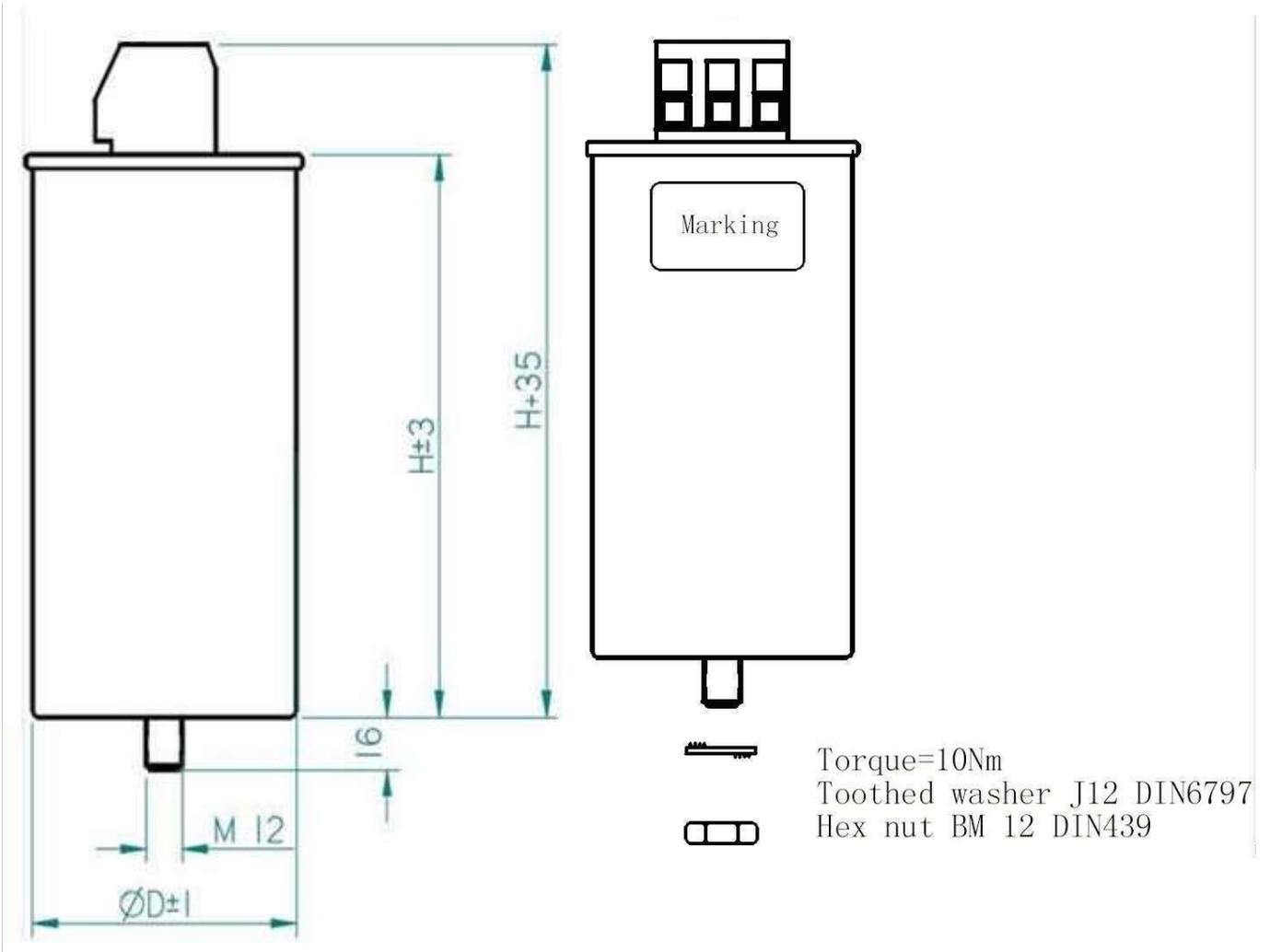
Max. cable cross section=25mm
