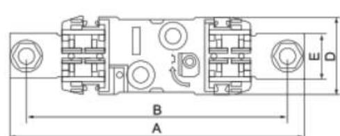
▪ Three phase Fuse base – Basic data & Dimensions/
